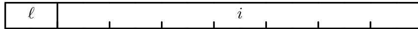
Figure 2.9: Layout of the unique node ID word U . The high-order byte is \ell , the level number. The seven-byte field i gives the index of the node within the level ( i = 0, 1, \dots ).
